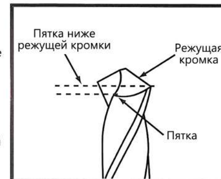
Figure 6. Heel must be lower than the cutting edge.
